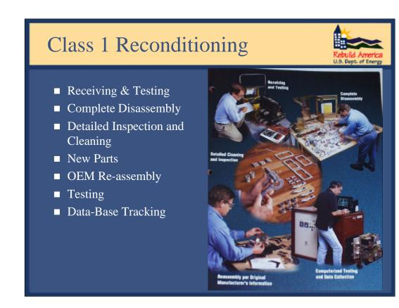
Even low voltage breakers can be brought to "like-new" condition using a technique known as "class 1 reconditioning". In this technology the circuit breaker is disassembled to its smallest parts. Each part is inspected. Parts out of tolerance are replaced and acceptable parts are cleaned. The breaker is reassembled, tested to the industry standards and warranted. This is an option if new breakers are not available and you don't want to replace the existing switchgear.
