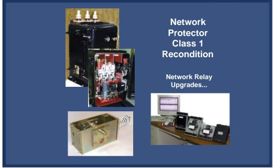
If you have a spot network, you will have network protectors. Old network protectors can be rebuilt with new switching elements and new network protector relays. These new relays substantially reduce the internal wiring, reducing the points of failure, while at the same time providing new diagnostics and protective settings to insure better operation of your spot network.
